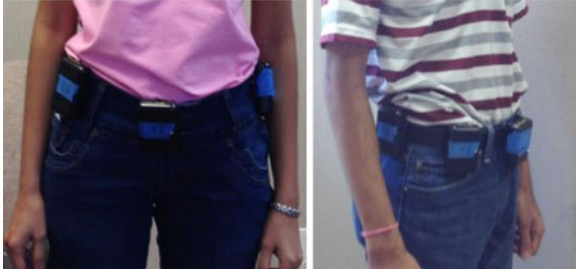
Fig. 4. Positions of three belt-clip accelerometers for feature selection.
